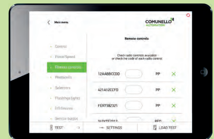
In Pro-settings the installer has complete management of up to 300 remote control codes.
